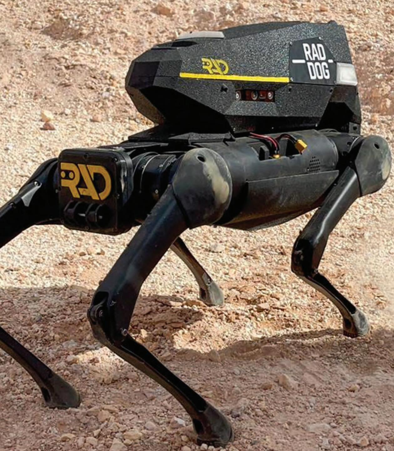
RADDOG 2LE, equipped with impressive capabilities that will exceed your expectations. With a maximum walking speed of up to 5 mph (2.23m/s), this agile robot can swiftly navigate any environment with ease. Its versatile maneuverability allows for quick runs, seamless backward steps, smooth lateral shifts, precise turning in place, subtle forward creeping, effortless rolling over, impressive jumps, obstacle crossing, and obstacle avoidance. Be prepared for the ultimate exploration experience.
